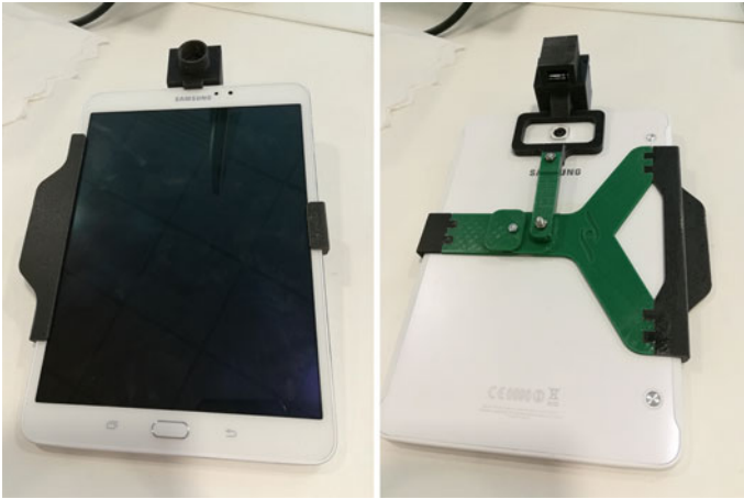
Fig. 6.6 Case of the ECOMODE camera: front, back
